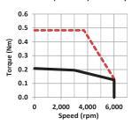
DC Bus--48VDC SM0402FE4(100 Watts) -5.2Amps
