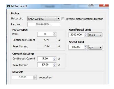
After setting the required parameters, click OK and then Download All to Drive to save the settings to the drive.
