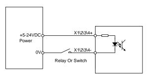
Sensor And Switch Connection
