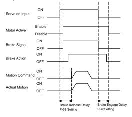
Brake engage/disengage delay time can be set through M Servo Suite software, or on the drive directly through the P function: P-69 (BD) or P-70 (BE).
