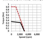
DC Bus--36VDC SM0401HE4(60 Watts) - 5.7 Amps
