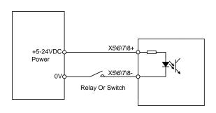
Sensor And Switch Connection
