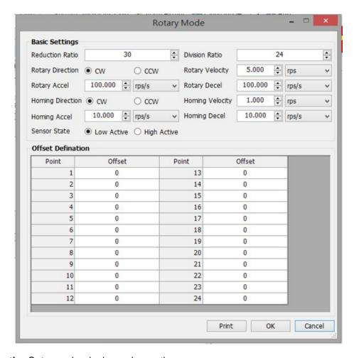
Reduction ratio: Sets mechanical gear box ratio
