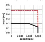
DC Bus--60VDC SM0402FE4(100 Watts) -5.2Amps
