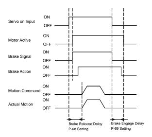
The Brake Output (BO) setting can be configured with the M Servo Suite siftware or with parameter P-67 (BO) as shown in the table below. Brake disengage delay and engage delay times can be configured via M servo suite software, or by changing parameters P-69 (BD) and P-70 (BE) directly on the drive.
