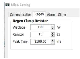
Wattage: The regeneration resistor wattage. M2DC drives calculate the continuous wattage induced into an external regeneration resistor and must know the continuous wattage rating of the regen resistor to do this effectively.
